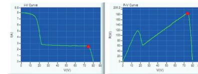
2.99.61% tracking efficiency in case of any shade in corners.
