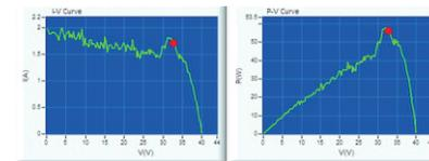
4.99.64% tracking efficiency in case of large area of shade.
